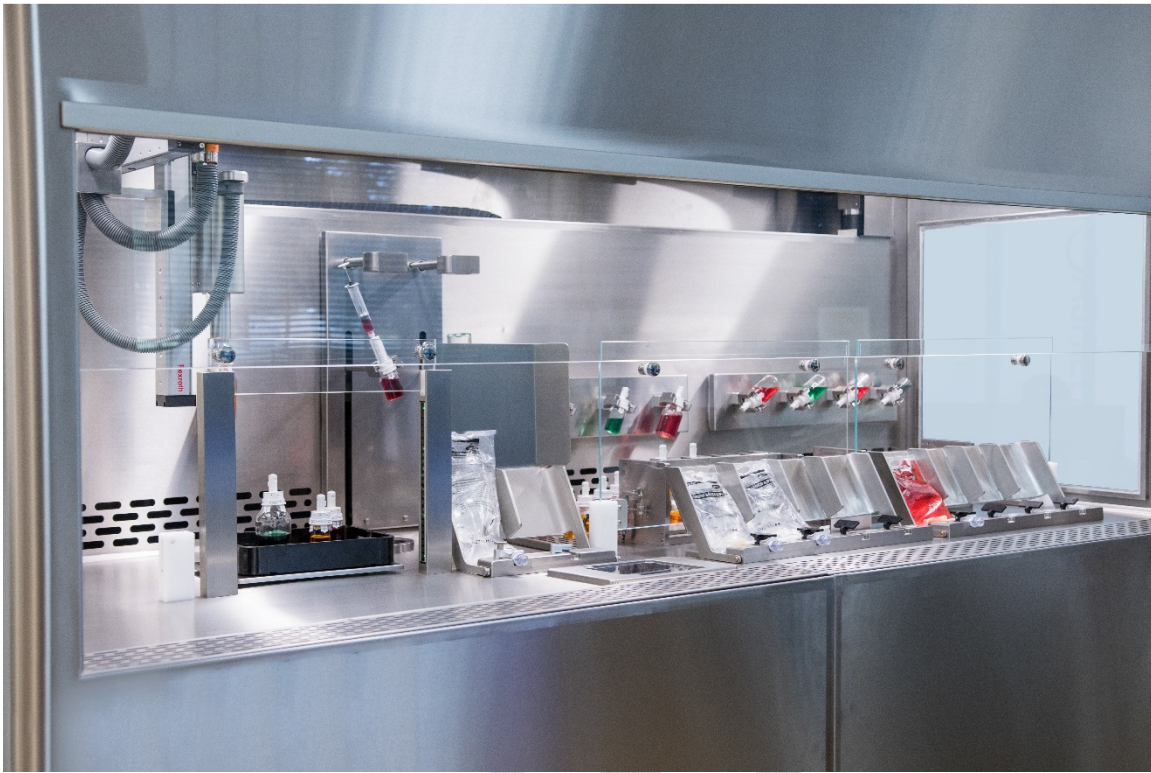
Figure 5. A robotic drug preparation system. Photo courtesy of Equishield.
