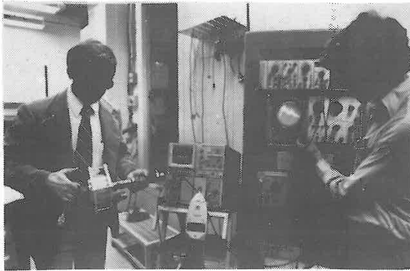
Figure 10. Anechoic Chamber and typical instrumentation used for acoustical measurement of an Ingersoll-Rand riveting gun.
