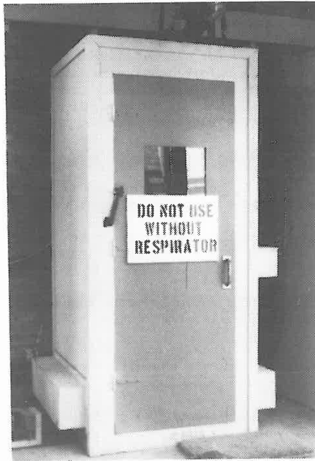
Figure 1. Outside view of downdraft booth. Air is exhausted from the booth through the lower protrusions on either side of the enclosure.
