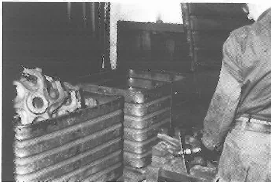
Figure 5. Bench grinding in small booth with exhaust capture behind bench. Note rubber flaps sealing booth opening.
