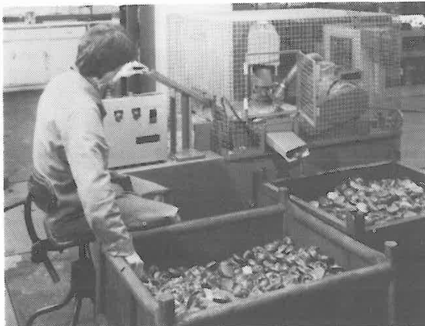
Figure 5. BCIRA designed machine for automatically grinding small circular castings.
