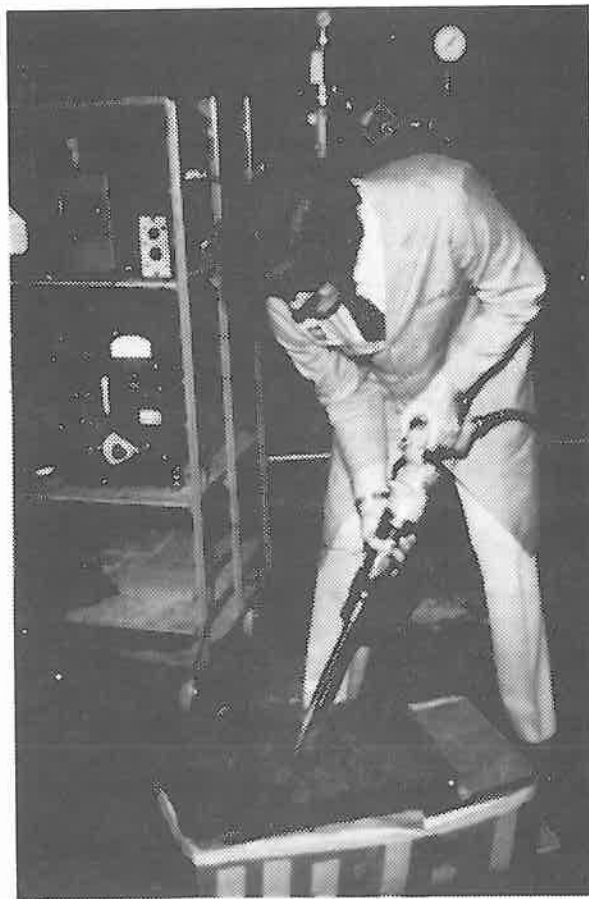
Figure 7. An experimental tool with a damped rubber isolator working in a non-resonant media.
