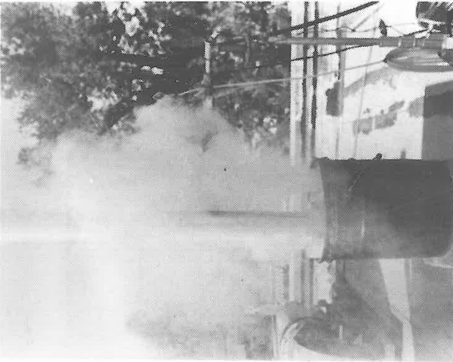
Figure 8. Dust boil-up during the free fall of dust into an open container (uncontrolled).
