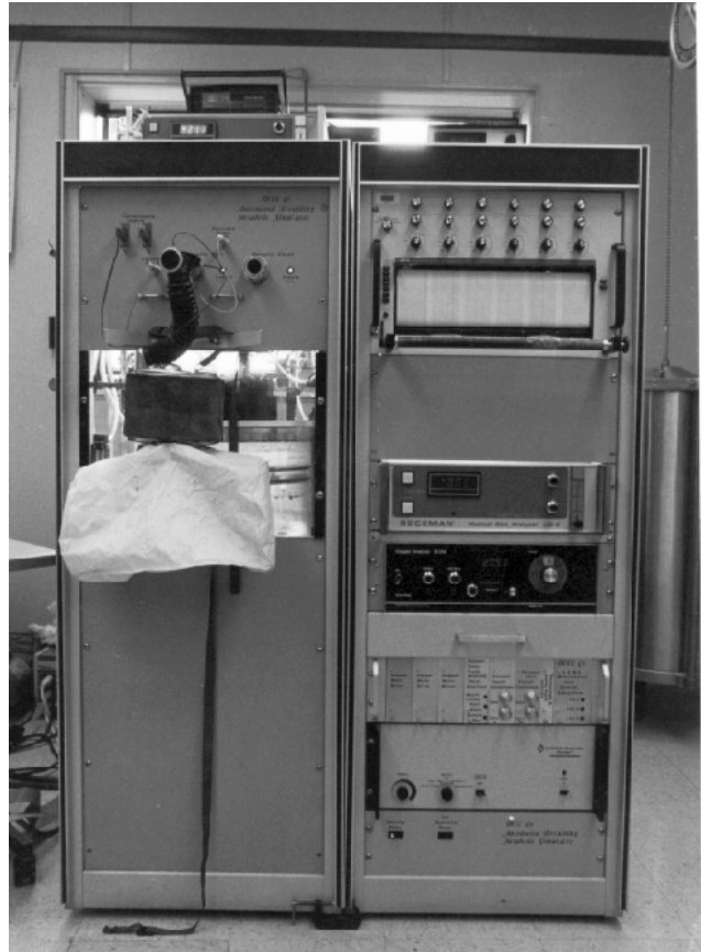
Figure 1.—Breathing and metabolic simulator (BMS) at the Pittsburgh Research Center, Bruceton, PA.
