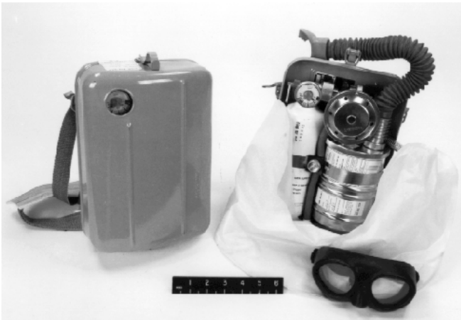
Figure 2.—Cased and uncased CSE AU-9A1 self-rescuer.
