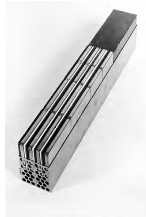
Figure 3. Typical Loaded ZPR Drawer.<sup>a</sup>
