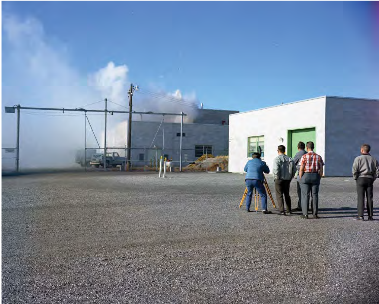
Figure 5-49: Smoke Test Performed as Part of the Building 626 Ventilation Checks
