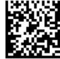
Figure 2: Example of two-dimensional barcode A two-dimensional, or data matrix, barcode can include product identification information as well as lot number and expiration date.
